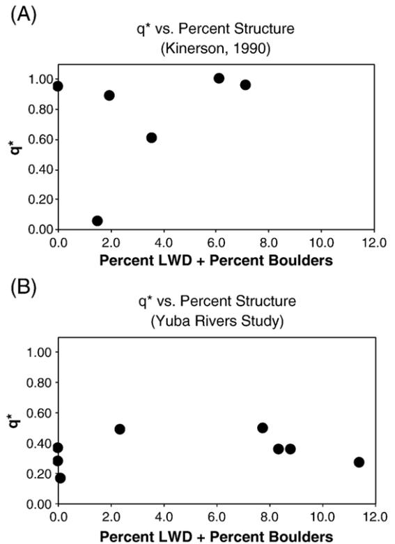
Fig. 8. Relationship between reach-averaged  $\bar{q}^*$  and percent area of structural elements for (A) Kinerson (1990) field study and (B) Yuba Rivers field study.
