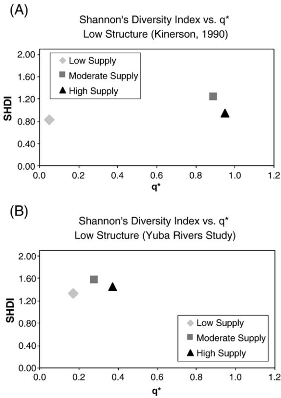
Fig. 9. Relationship between relative sediment supply ( $q^*$ ) and geomorphic diversity (SHDI) in reaches with <2% structural elements for (A) Kinerson (1990) field study and (B) Yuba Rivers field study.
