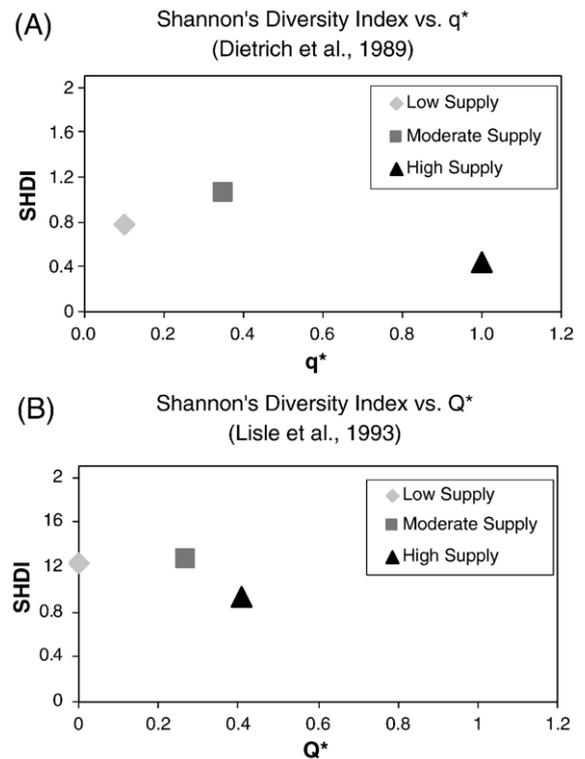
Fig. 5. Relationship between relative sediment supply ( $q^*$  or  $Q^*$ ) and geomorphic diversity (SHDI) for (A) Dietrich et al. (1989) flume study and (B) Lisle et al. (1993) flume study.
