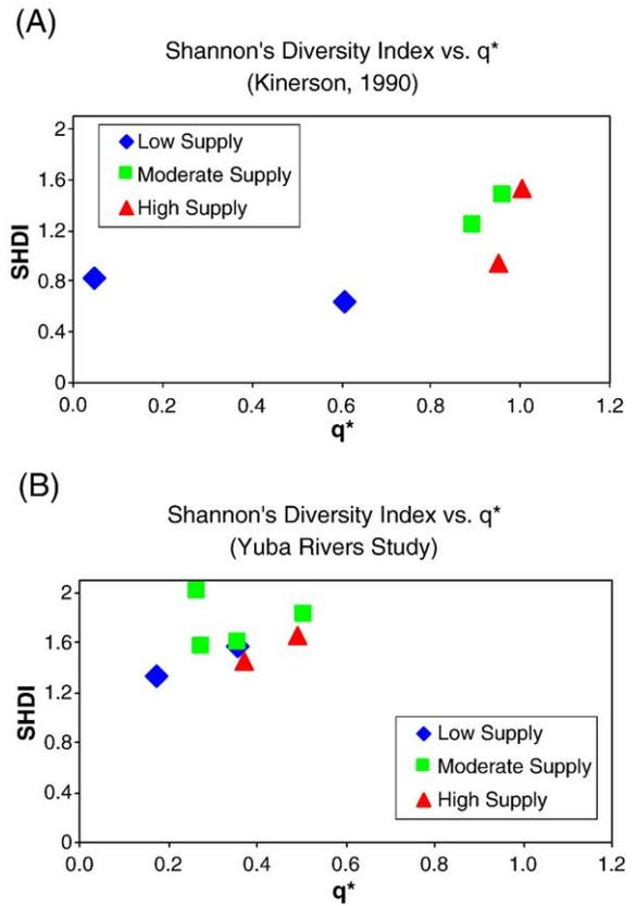
Fig. 6. Relationship between relative sediment supply ( $\bar{q}^*$ ) and geomorphic diversity (SHDI) for (A) Kinerson (1990) field study and (B) Yuba Rivers field study.
