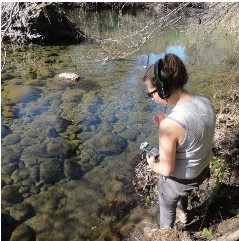
Figure 3: Recording underwater vocalizations of Rana boylei in the Big Chico Creek Ecological Reserve. The hydrophone is underwater and the Zoom H4n recorder is being held.
