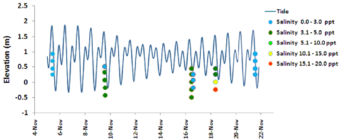
Figure 12. Tide height and salinity measurements through the water column at TEM-MOL. Salinity measurements show temporal variations throughout the study period. Salinity measurement were usually well mixed and between 0-5 ppt, however on one day there was a halocline and the two deepest measurements were above 10 ppt. Looking at tide data, the relationship between tides and salinity is not clear.
