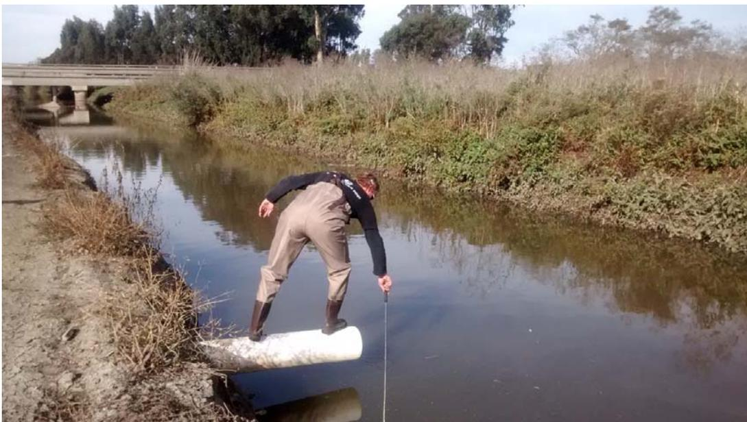
**Figure D2:** At the Haro St. sample site we collected the turbidity sample off of the end of a drainage pipe to get access to the mid-channel water.
