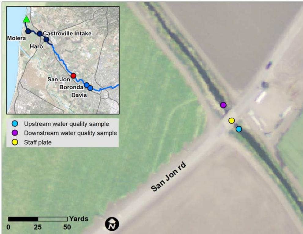
Figure C7: Map of the San Jon Rd. sample site. The pygmy meter measurements were taken midway up the concrete channel upstream of the USGS staff plate. Float measurements were started approximately 20 ft upstream of the staff plate and ended just above the staff plate.
