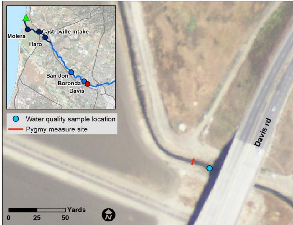
Figure C11: Site map of the Davis Rd. sample site. Water quality samples were taken downstream of a hydraulic jump caused by an obstruction in the water channel. The streamflow measurements were also taken downstream of the hydraulic jump.
