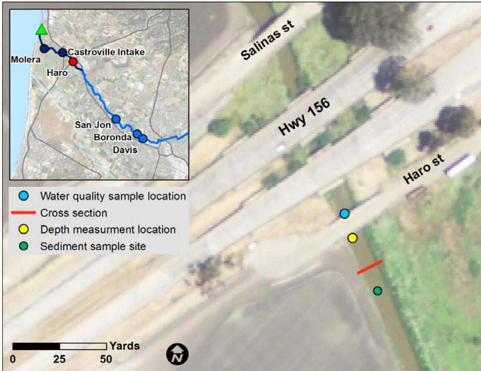
Figure C5: Map for the Haro St. sample site. Sediment samples were taken off the end of the tile drain located south of the Haro St. bridge. Depth measurements were taken off the bridge by lowering a stadia rod into the water and reading the depth from the bank. All measurements were relative and tied to the cross section.
