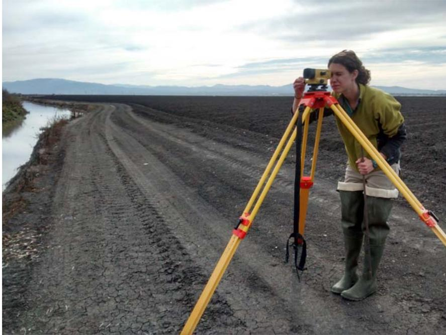
**Figure D1:** We used an auto level to measure the cross-section at the Haro St. and Molera Rd. sample sites. This photo was taken at the Haro St. site, upstream of the bridge.
