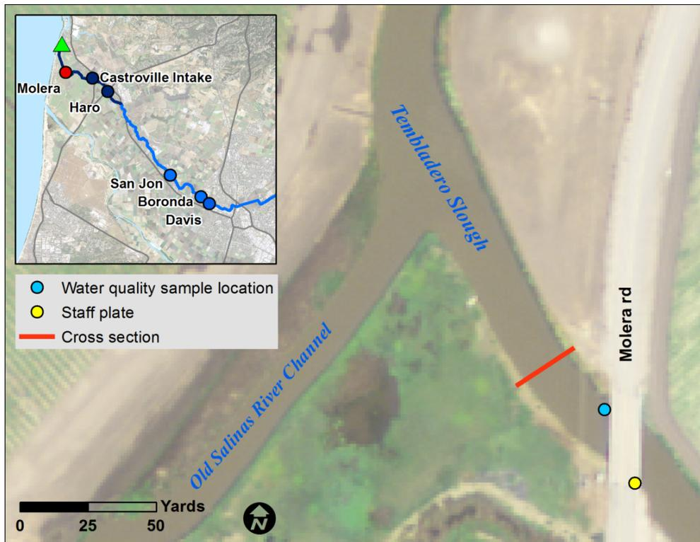
Figure C1: Site map for the Molera Rd. sample site. The staff plate is located under the bridge on the south east side. Streamflow measurements were taken downstream of the observed turbulence from the Molera Rd. bridge, and upstream of the confluence with the Old Salinas River Channel.
