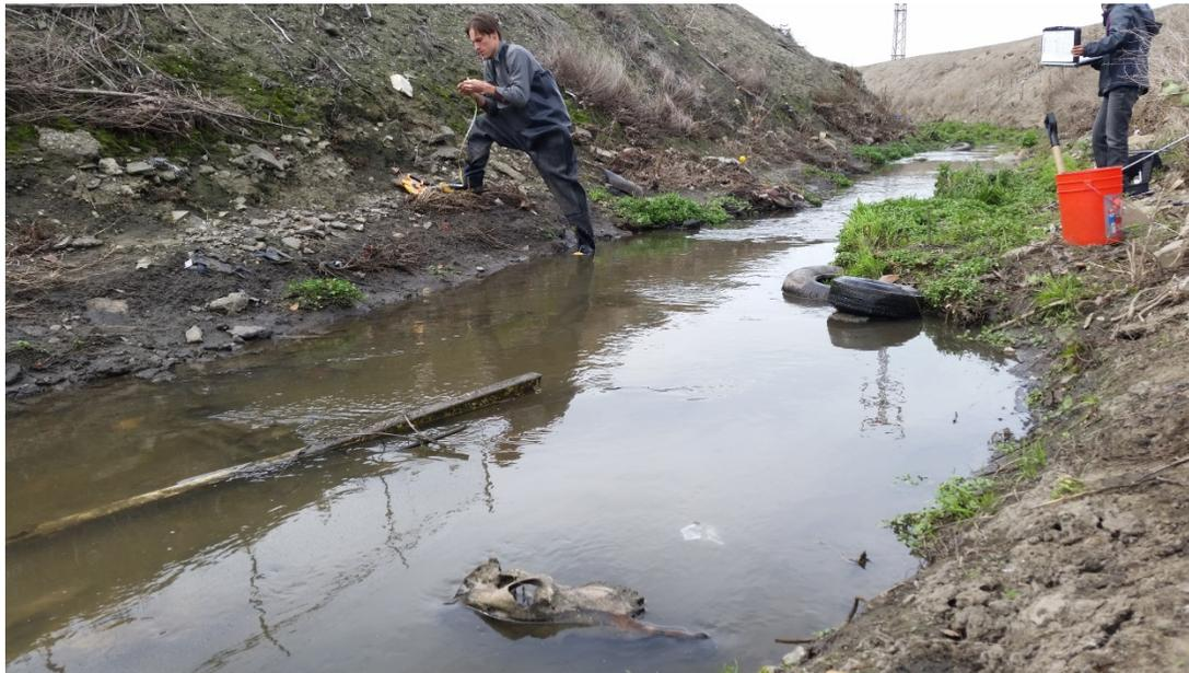
Figure C10: Preparation for pygmy meter measurements at the Boronda St. sample site. We made some minor bank alterations to improve the quality of the pygmy measurements.
