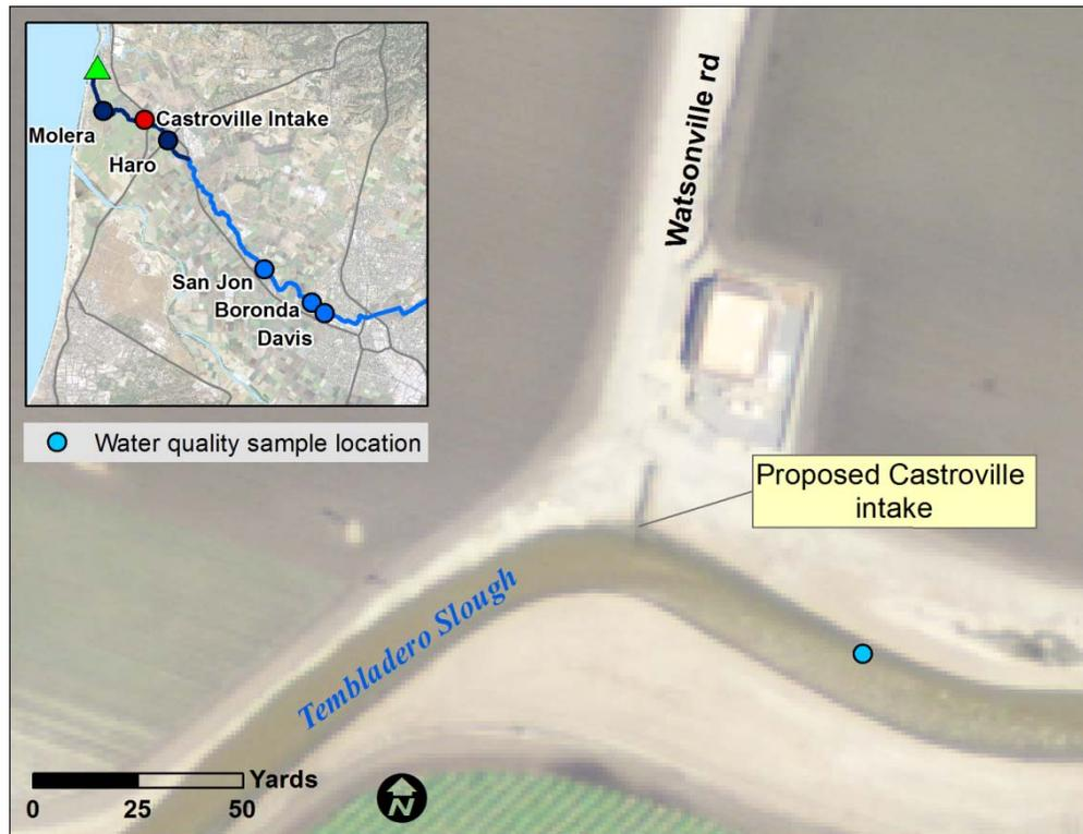
Figure C3: Map for the Castroville Intake sample site. Water quality measurements at the Castroville site were taken from the bank. We observed that at this location the slough had a trapezoidal cross section with a flat uniform bottom with no obvious thalweg for taking measurements. The lack of a stable structure to take consistent depth measurements prevented us from collecting streamflow data.
