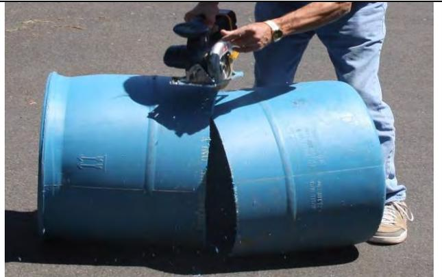
Figure 12. Cutting barrel in half with skillsaw.
