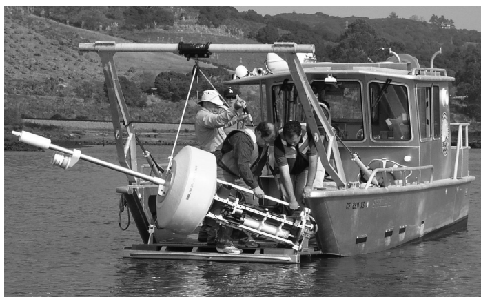
Fig. 6. A vertical mooring, L02, being deployed with RV Sheila B.
