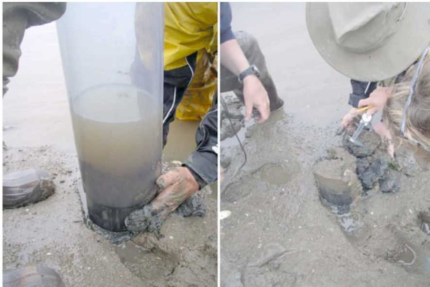
Fig. S2. Sediment cores taken to measure the aRPD
