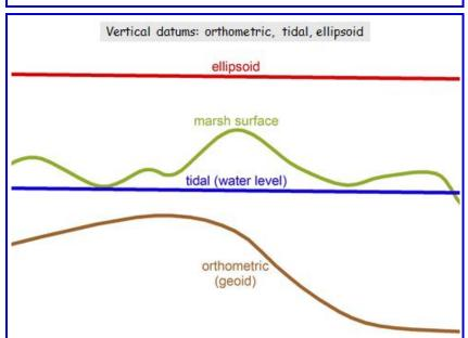
Reconciling three types of elevation measurements (vertical datums) is necessary to produce a DTM and water surface suitable for sea level and marsh sustainability modeling.
