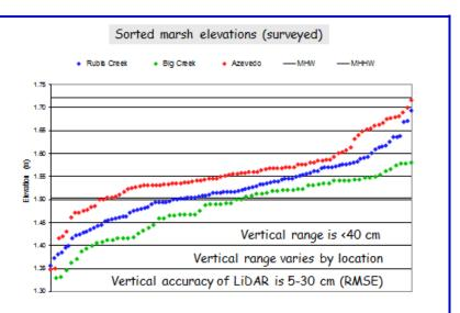
LiDAR elevation data, adjusted to account for tidal variability, barely provides the required vertical accuracy.
