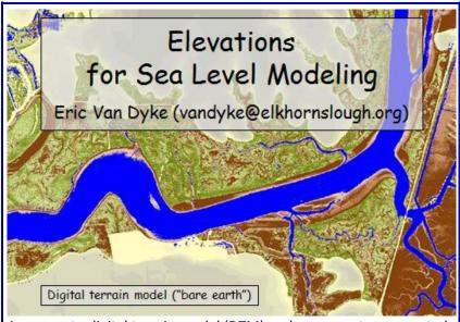
An accurate digital terrain model (DTM) and an accurate, connected water surface are essential for modeling sea level rise and marsh sustainability.
