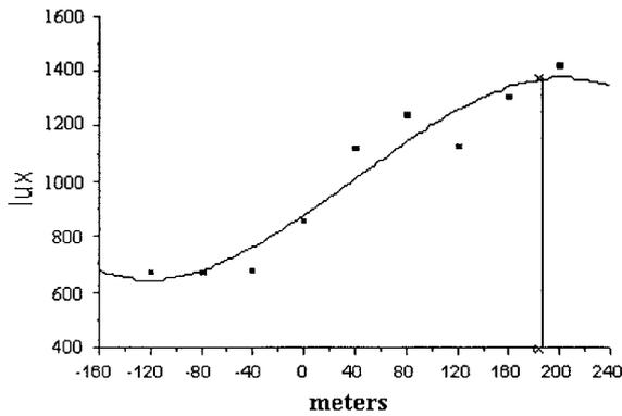
Figure 2. Solar radiation and distance from the edge measured across timber harvest boundaries in Redwood National and State Parks ( $R^2 = 0.242$ ,  $p < 0.0001$ ). Depth of influenced estimated using a procedure adapted from Oosting (1948). The scale on the  $x$ -axis refers to distance from the edge as positive in the direction of the old-growth forest and negative in the direction of the regenerating areas. The zero mark represents the timber harvest boundary.
