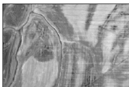
C9 – Saturation visible on aerial imagery (Secondary)
